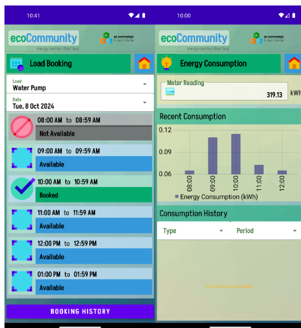
Figure 51 Screenshots of flexible load booking use case in Gaidouromandra demo site (Left) consumer interface showing the booking details (Right) consumer consumption during the booked period
