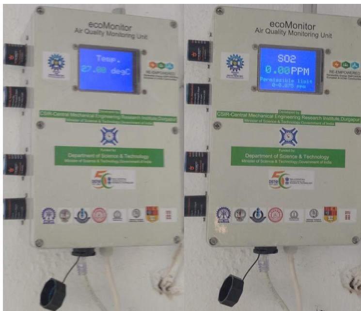
Figure 47 Real time monitoring of air quality parameters SO 2 (left) and Temperature (right).
