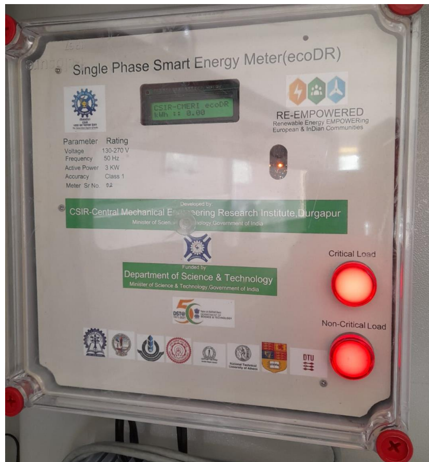
Figure 37 : ecoDR demonstrating energy consumption (as nil) of non-critical load when load scheduling command received from ecoMicrogrid
