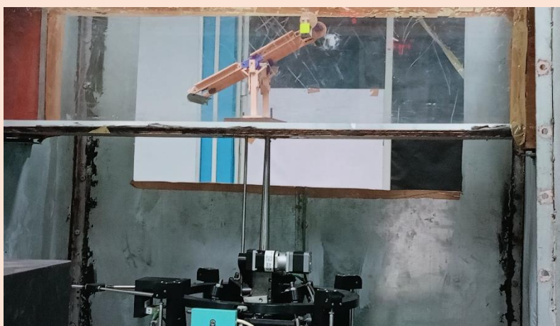
Fig. A16 Wind tunnel testing of 1:10 scale down models of solar PV support structures
