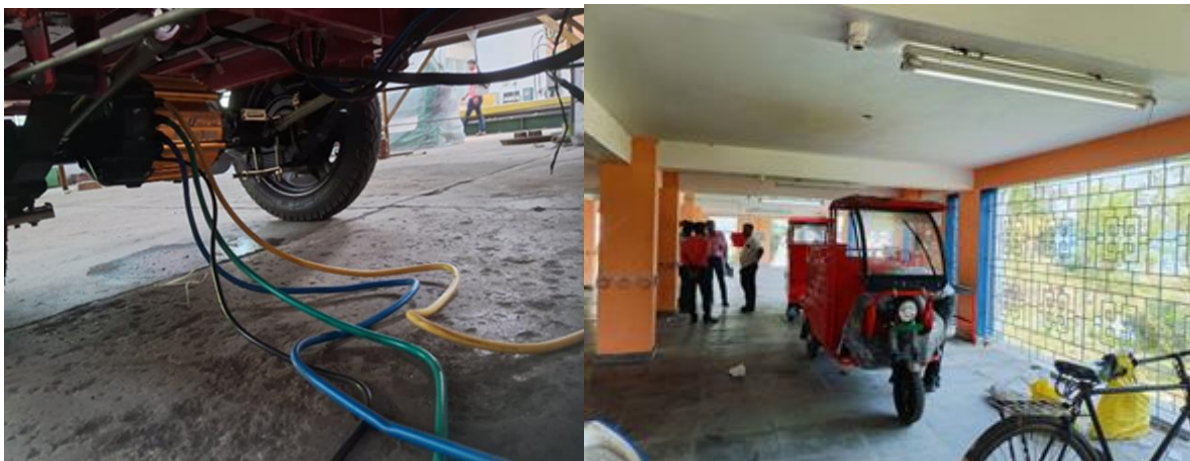
Figure 127 Electric three-wheeler powertrain upgraded to 2 kW BLDC motor with matching controller and (right) deployment at Ghoramara demo site
