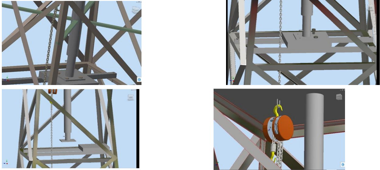
Figure 116 Fixing of monopole over the truss structure for power generation & lowering of tower during cyclone using a chain hoist having a capacity of 1 ton.
