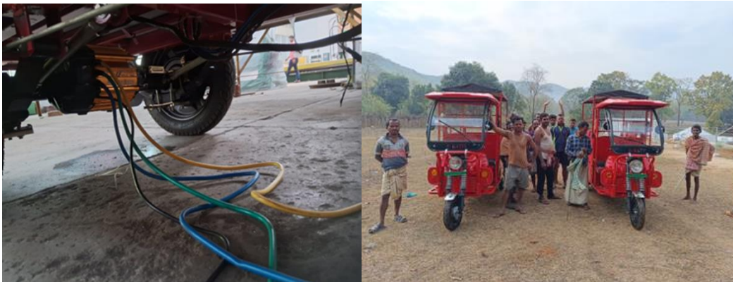
Figure 162 Electric three-wheeler powertrain upgraded to 2 kW BLDC motor with matching controller and (right) deployment at Keonjhar demo site
