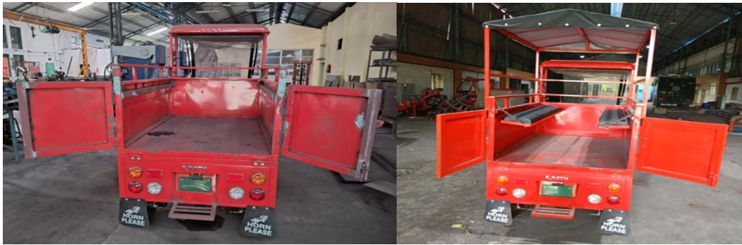
Figure 163 (Left) Electric three-wheeler converted into an electric loader to transport goods (seating arrangement and canopy removed) and (right) modular seating arrangement and canopy for carrying passengers.
