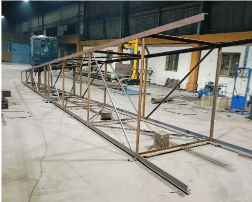
Figure 117 Making of foundation and fabrication of hybrid tower as the final drawings
