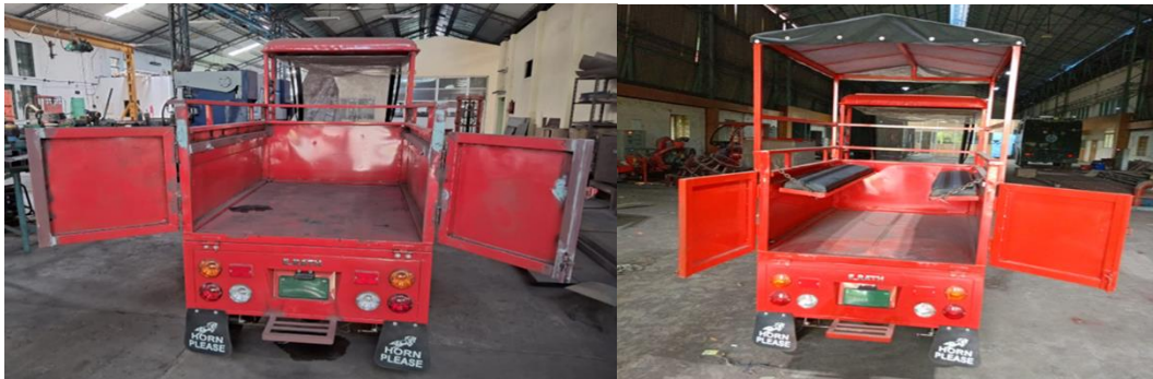
Figure 126 (Left) Electric three-wheeler converted into an electric loader to transport goods (seating arrangement and canopy removed) and (right) modular seating arrangement and canopy for carrying passengers
