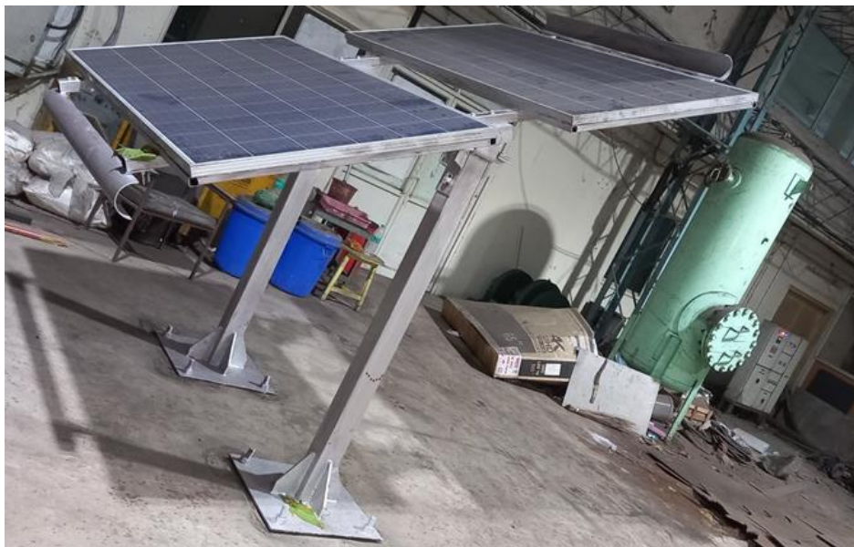
Figure 110 Final fabricated prototype of the solar PV support structures that is being installed at Ghoramara demo site.
