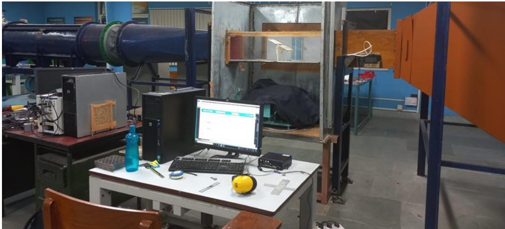
Figure 108 Wind tunnel testing of solar PV with support structure. Aerodynamic loads on support structure are examined using a load cell.
