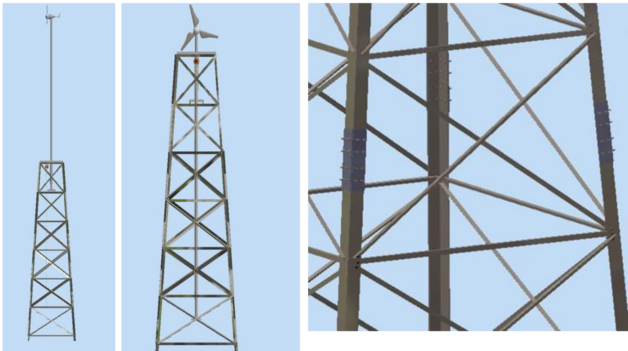
Figure 115 Power generating position (18 m) and rest position (12 m) during cyclone. Each component of the truss structures is connected through nuts & bolts
