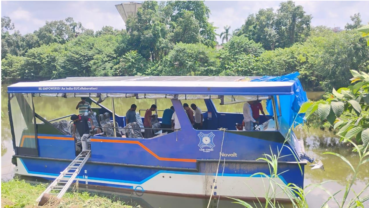
Figure 128 Rooftop solar PV integrated electric boat for mainland connectivity
