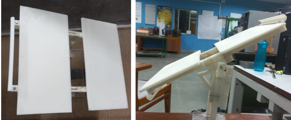
Figure 107 1:10 Scale-down model of the support structure with PV panels
