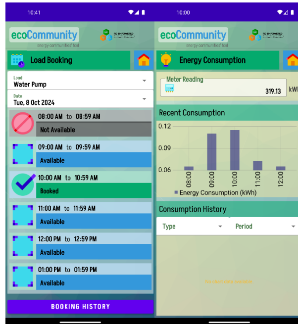
Figure 81 Screenshots of flexible load booking use case in Gaidouromandra demo site: (Left) consumer interface showing the booking details. (Right) consumer consumption during the booked period
