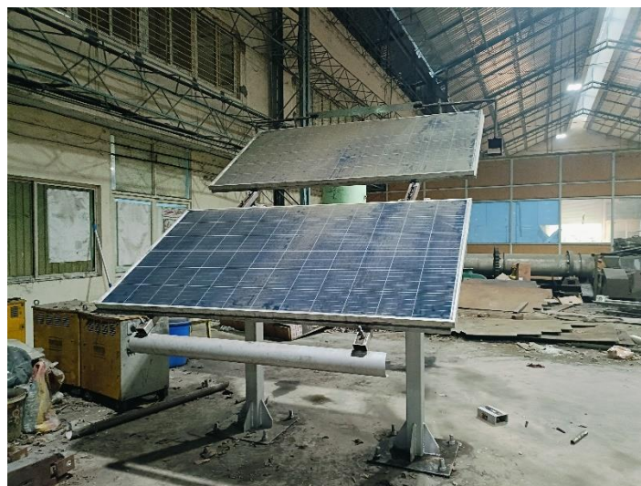
Figure 23: Tested support structure with passive add-on aerodynamic components for Solar PV to reduce aerodynamic loads due to cyclone: at CSIR-CMERI premises.
