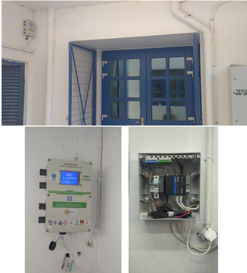
Figure 51: ecoMonitor deployment at the school of Kythnos and its communication router panel.
