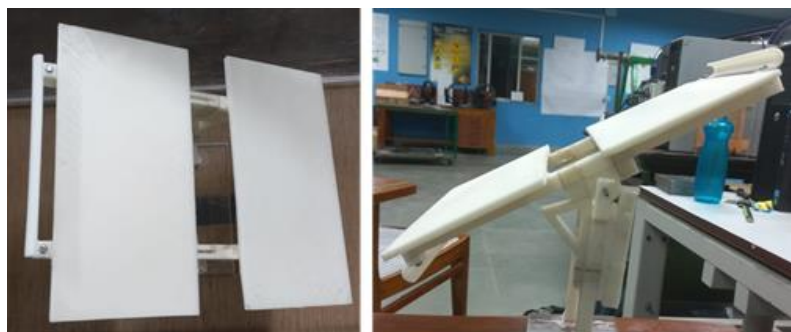
Figure 78: Scale-down model of the support structure with PV panels
