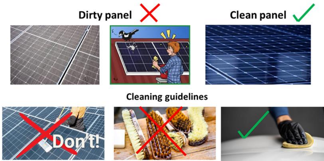
Figure 55. Training of how to clean the panels.
